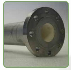
Carten Ceramic spools are utilised to protect customer systems where abrasion can be at it's highest level – post the control valve installation, where high-velocity media streams can cause high levels of wear. This protects the customer core piping system with our 95% Alumina ceramic, and can be assembled without disrupting the pipelines
