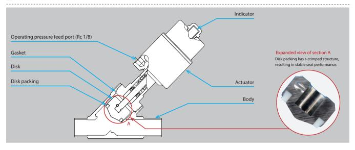
Actuator can turn 360°, allowing adjustment of orientation of operating pressure feed port.
